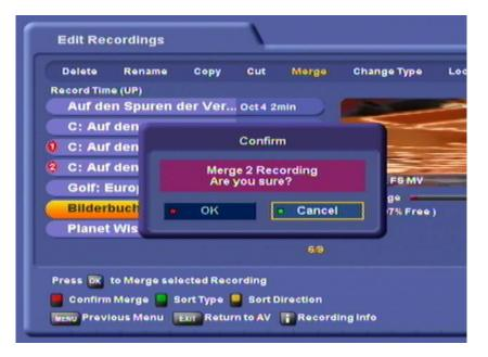
Use the buttons to select "OK" and press to start merging the recordings. The receiver merges the two recordings. The newly created single recording is assigned the name of the first recording you selected for merging.
